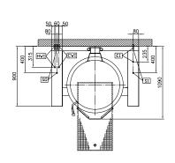
Electric Supply voltage: 230 V/1N ph/50/60 Hz Total Watts: 0.2 kW Steam Steam generation: External source Steam inlet size: Steam pressure Max: 1.5 bar Steam supply, relative 1 min bar, 1.5 max bar dynamic pressure: Water: Pressure, min-max: 2-6 bar Installation: FS on concrete base;FS on feet;On base;Standing Type of installation: against wall **Key Information:** 50 °C **Working Temperature MIN:** 110 °C **Working Temperature MAX:**
